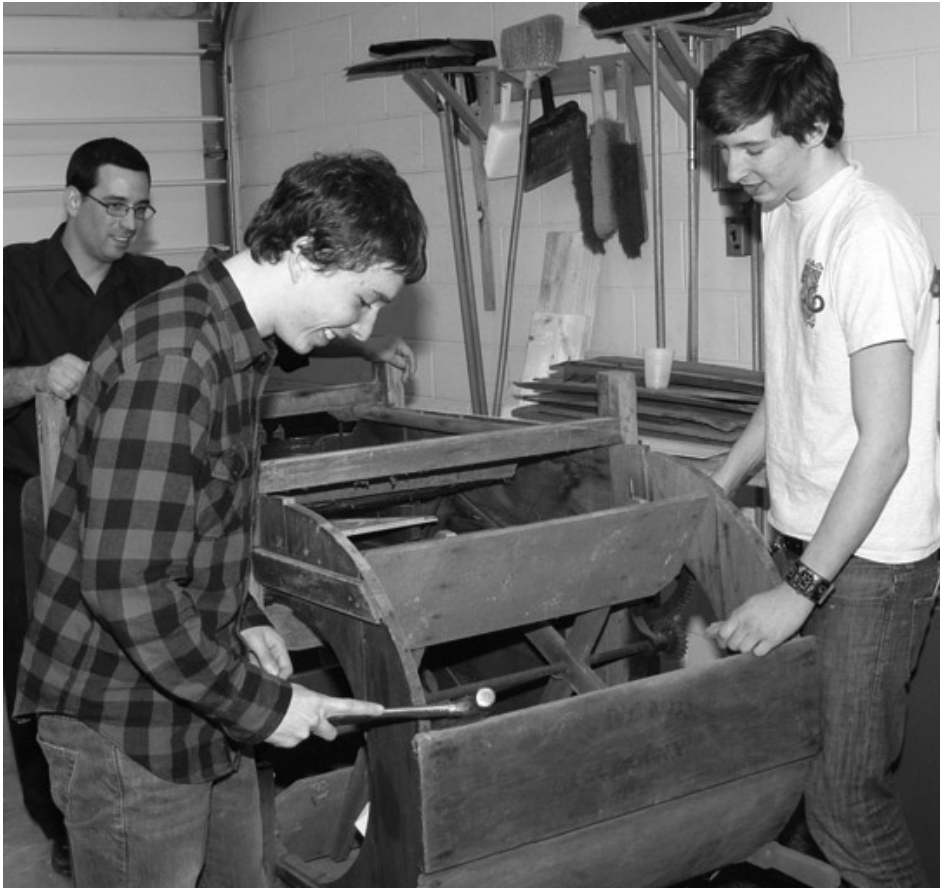
Austin Halligan (left) and Jessie Creighton (right) work on refurbishing a fan mill, which was used in the late 1800's to separate grain. The fan can be powered by the saw mill when complete. Over seeing the project is instructor Rico Ruffino at Iroquois Woodworking Technology classes.
